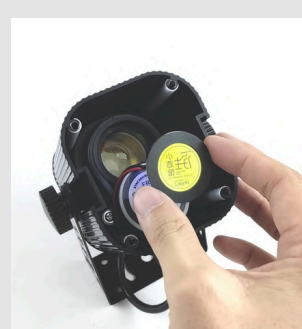
Step 3: Install new GOBO and snap ring,the GOBO need the reverse side up.
