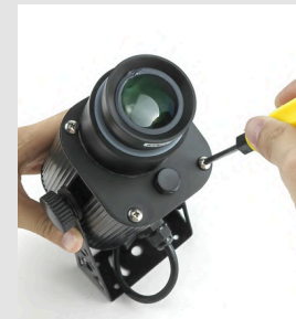
Step 1: Screw out all the screws of the front cover of the machine.
