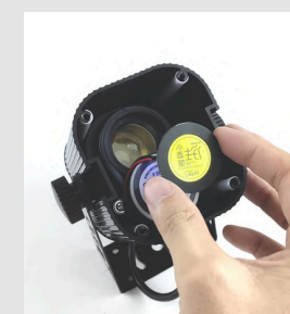
Step 3: Install new GOBO and snap ring, the GOBO need the reverse side up.
