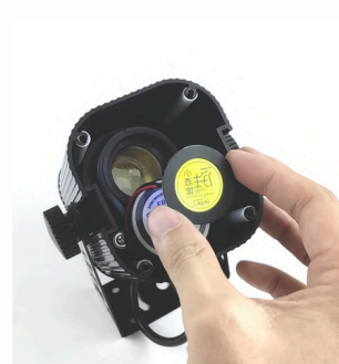
Step 3: Install new GOBO and snap ring,the GOBO need the reverse side up.
